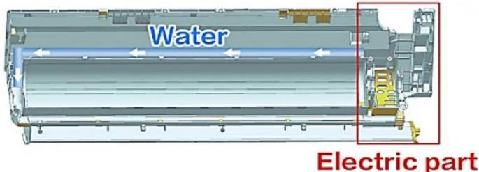
No connection between condensate water and electricity
